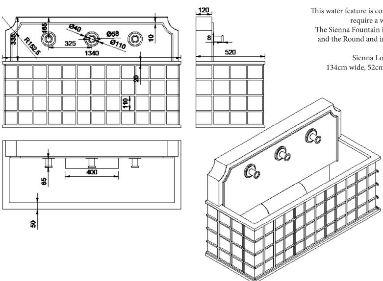
This water feature is completely self contained, so you will not require a water supply to the feature.
